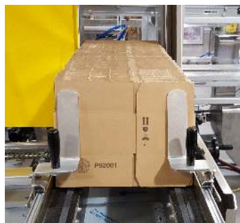
Ergonomically Designed Large Capacity RSC Case Magazine
