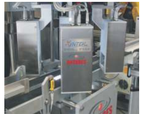
Infeed Conveyor with Track & Trace Serialization Cameras for Aggregation
