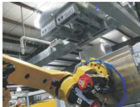
Integrated Overhead Vision System Verifies Case Load
