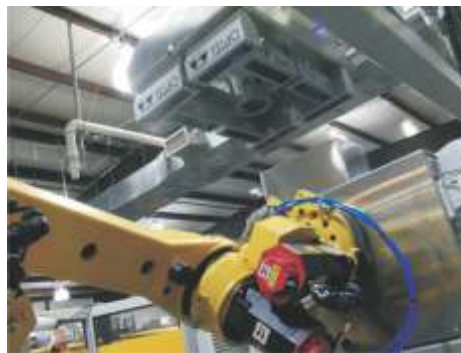
Integrated Overhead Vision System Verifies Case Load
