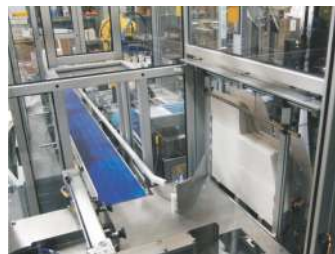
Carton Conveyor to Loader
