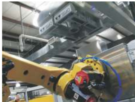
Integrated Overhead Vision System Verifies Case Load
