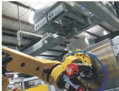
Integrated Overhead Vision System Verifies Case Load
