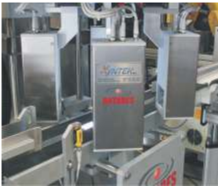
Infeed Conveyor with Track & Trace Serialization Cameras for Aggregation
