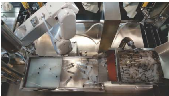
Flex Feeder for Syringes with LR200iD Clean Class Robot
