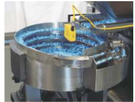
Cap feeders can be centrifugal or vibratory, depending on the required specifications.
