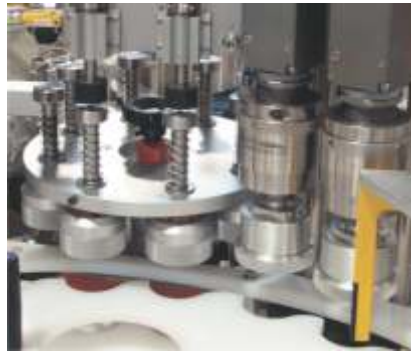
Unique, reliable capping device applies the cap, and final torque is accomplished using a stainless steel magnetic clutch torque head.
