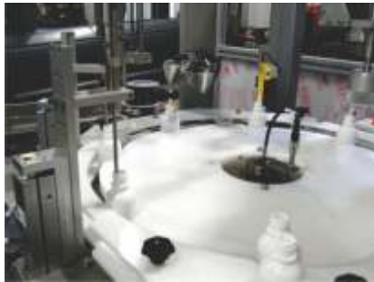
Two filling stations, plug inserter station & plug inspection.
