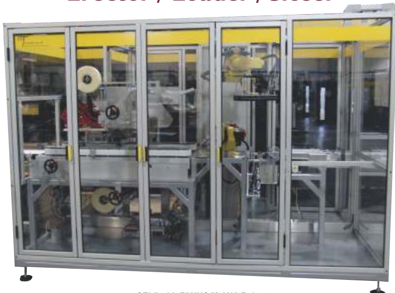
CEL5 with FANUC M-10iA Robot
