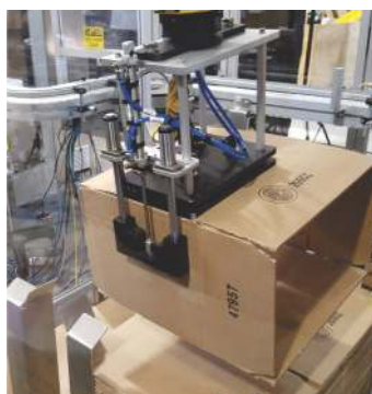
Erecting an RSC Case
