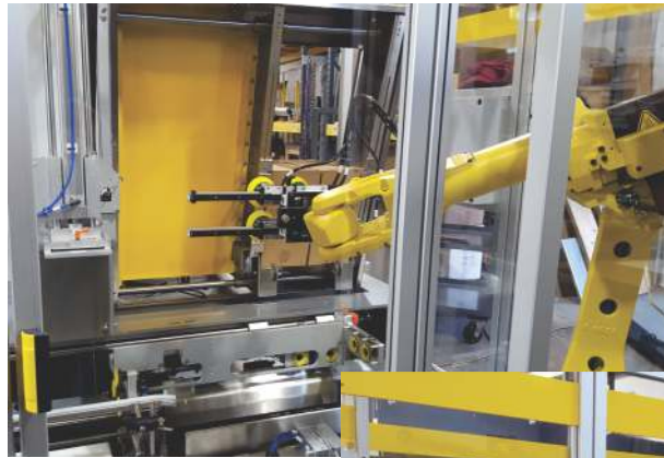
CE15 Case Erector with FANUC M-10iA Robot
