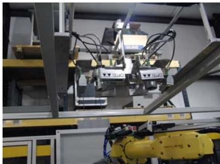
Overhead Camera Integrated with a Robotic Case Packer
