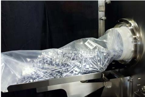
Bag of Sterile Syringes Connected to RTP
