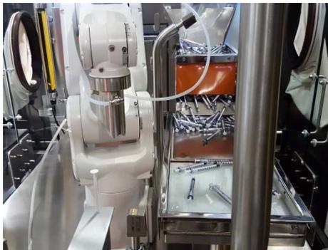
Robotic Flexible Feeding System for Syringes
