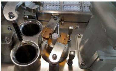
Capping Station and Discharge / Reject Chutes
