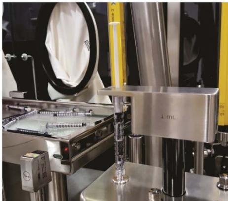
Filling Station on Model SF20 TaskMate® Aseptic Syringe Filler and Capper
