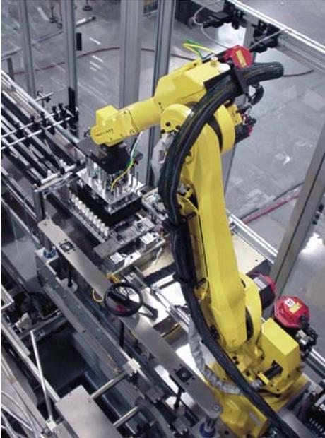
FANUC M-16iC Robot in a Vertical Case Packer Application
