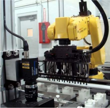
**Integrated Vision for Inspection of Diagnostic Test Kits**
