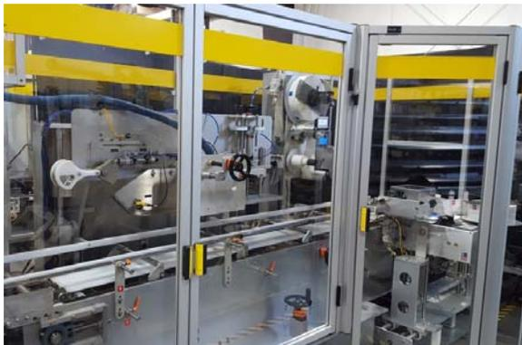
To meet serialization requirements for pharmaceutical manufacturers, ESS works with serialization system OEMs to seamlessly integrate coders, labelers, and inspection systems to create a solution for track-and-trace case packing applications. ESS has installed dozens of serialization-enabled case packers in North America and
