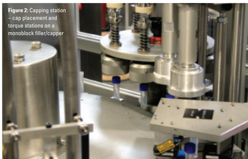
**Figure 2:** Capping station – cap placement and torque stations on a monoblock filler/capper
